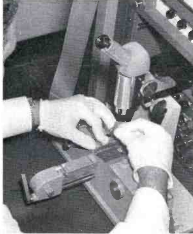
FIG. 8. Again the shear type cutter is brought in position and another cut is made.
