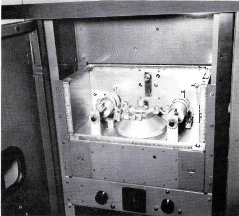
FIG. 5. The single 4CX1000A PA stage is shown here. The input and output tuning coils are shown on each side of the tube. The shield cover is easily removed to provide easy access to the stage, especially for tube replacement.
