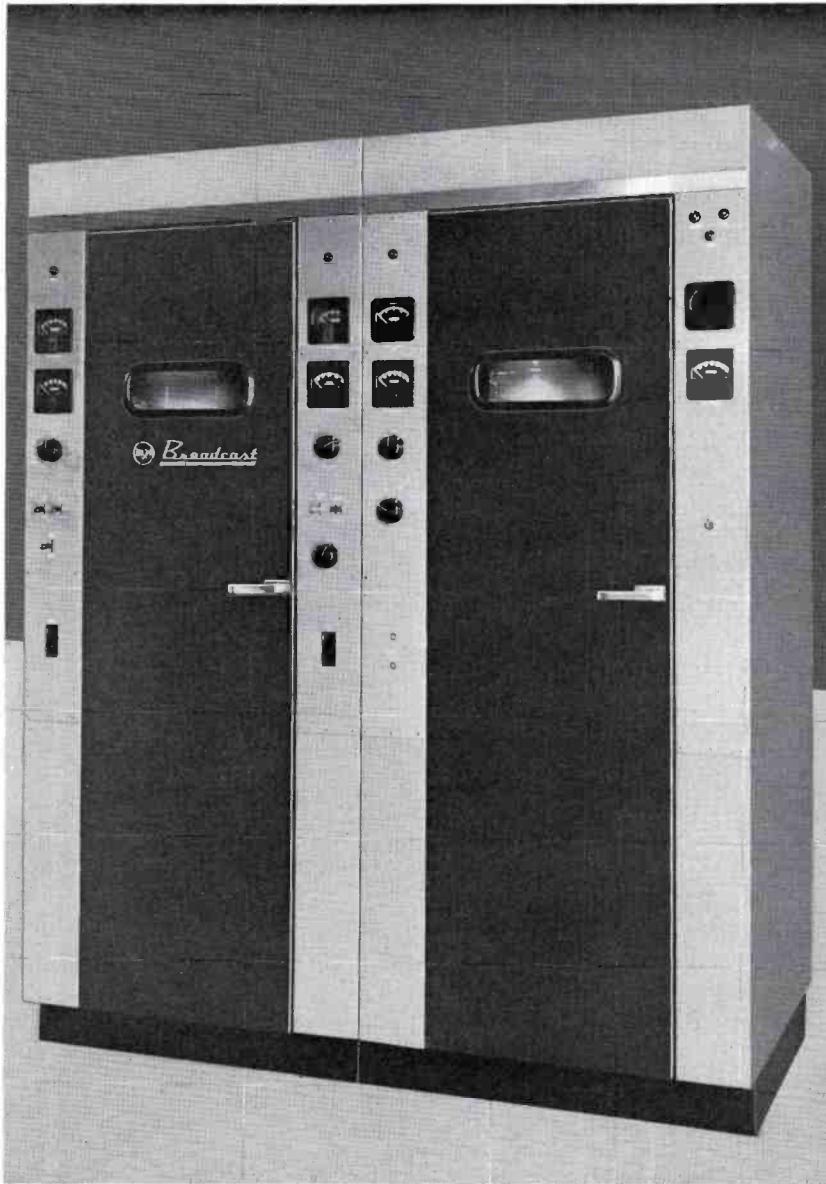
FIG. 1. Easy access to all tubes is made through two interlocked front doors of the BTA-5T Transmitter. The PA, modulator, and silicon rectifiers are in the cabinet on the right, and the exciter, driver and control equipment is on the left. The attractively styled cabinets are available with red or gray doors.
