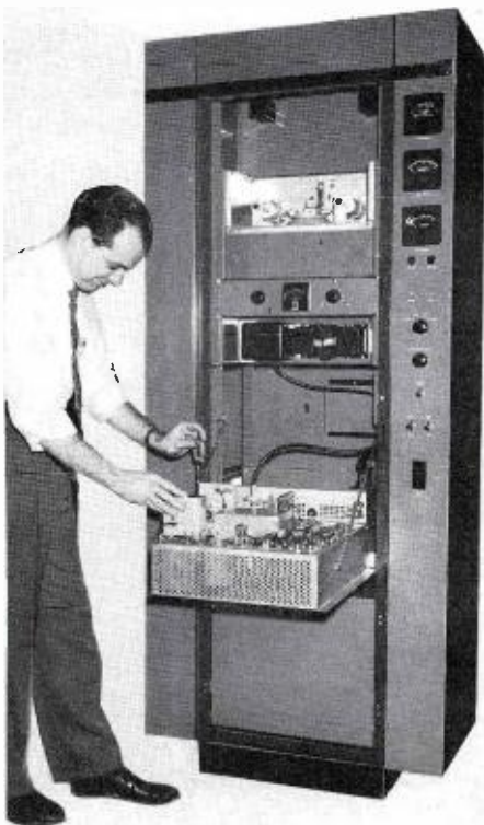
FIG. 2. The author is shown demonstrating the accessibility of the BTE-10B Exciter which tilts out for servicing.
