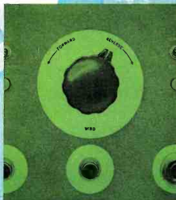
Variable Speed Cuing Control
