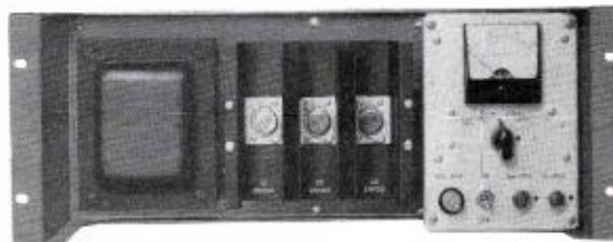
FIG. 6. Completely transistorized, the WP-16 power supply provides all power needed for operation of the camera chain.
