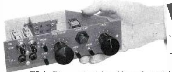
FIG. 5. This compact control panel houses the remote iris control, a combination gain and pedestal "mood effects" control, preset gain and pedestal controls, electronic lens cap switch and intercom phone jacks and level controls.
