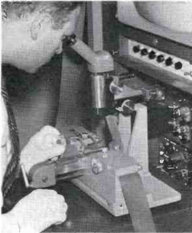
FIG. 7. The tape track is again aligned prior to making the precision cut necessary to match the two ends of the tape.
