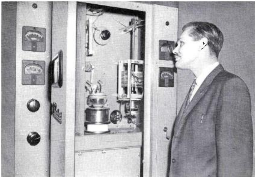
FIG. 4. The author is shown adjusting the new PA stage. Only one 5762 tube is used for high efficiency operation. The coil, shown on the right is the third harmonic coil used in the plate circuit of the PA to increase efficiency by shaping the plate waveform
