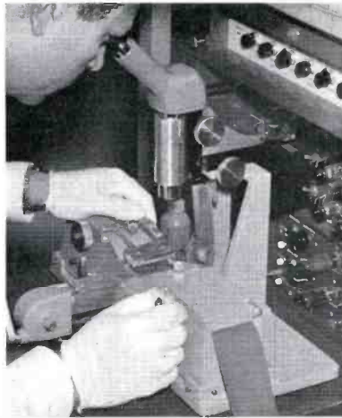
FIG. 4. The edge of the video track is lined up on the reticle built into the microscope. When properly aligned, the shear type cutter will cut the tape half-way between adjacent video track.
