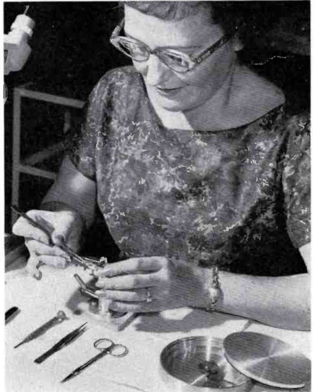
FIG. 6. After machining, the two halves of the magnetic head are cemented together using a special fixture. At this point the gap spacer is inserted between pole tips. The gap spacer is hardened beryllium copper foil rolled to a thickness of less than 0.000095 inches.
