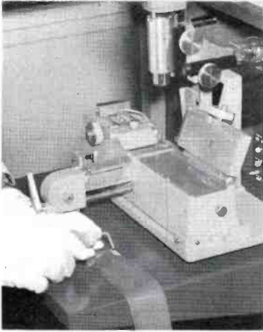
FIG. 3. The nearest "edit" or "frame" pulse is located by dispensing a liquid solution of iron oxide particles on the tape. This develops the magnetic pattern.
