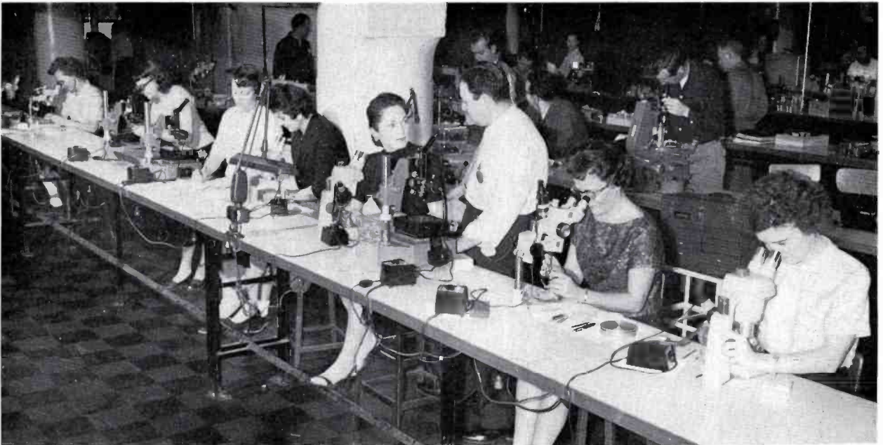
FIG. 4. The tiny components of the TV Tape magnetic head are assembled on production lines such as this. Operators work in a world of powerful magnification, inserting pole tips into head blocks, wiring tiny cores, assembling the various components which make up the completed magnetic head.
