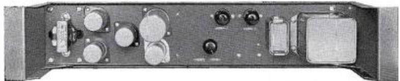
FIG. 1. Automatic sensitivity control is a 3½-inch rack mounted chassis.
