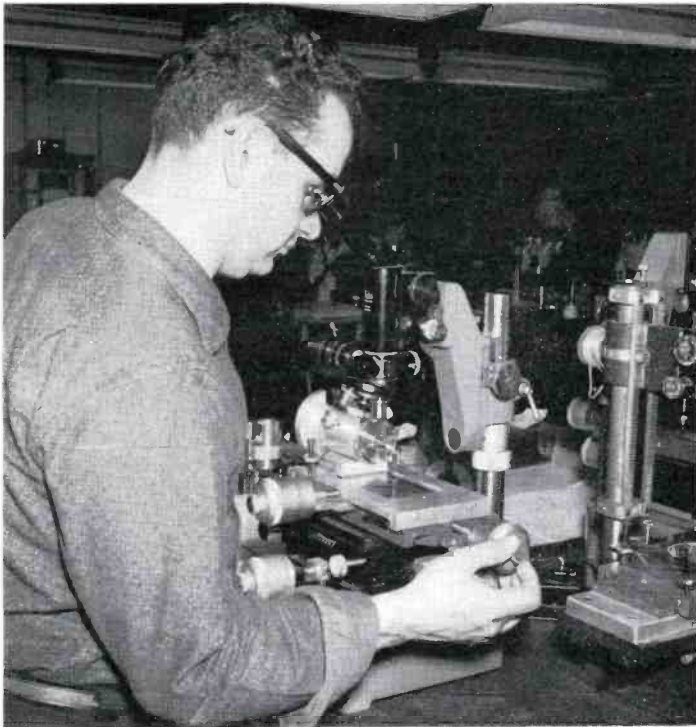
FIG. 7. Individual heads are placed in special alignment fixtures, and accurately set with respect to pole-tip protrusion, tracking, quadrature and balance. Once rigid specifications have been met, the heads are transferred and cemented to the headwheel assembly.
